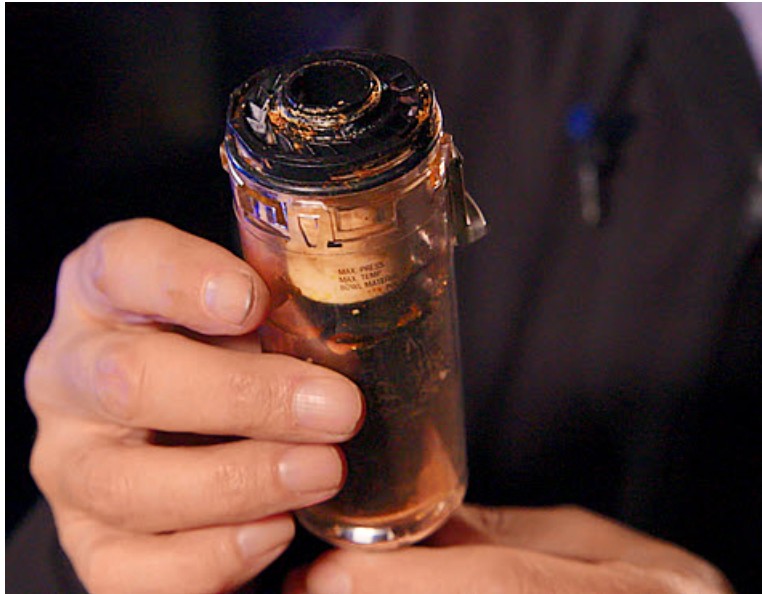
Figure 5 - Example of a dirty air filter bowl (continued)
